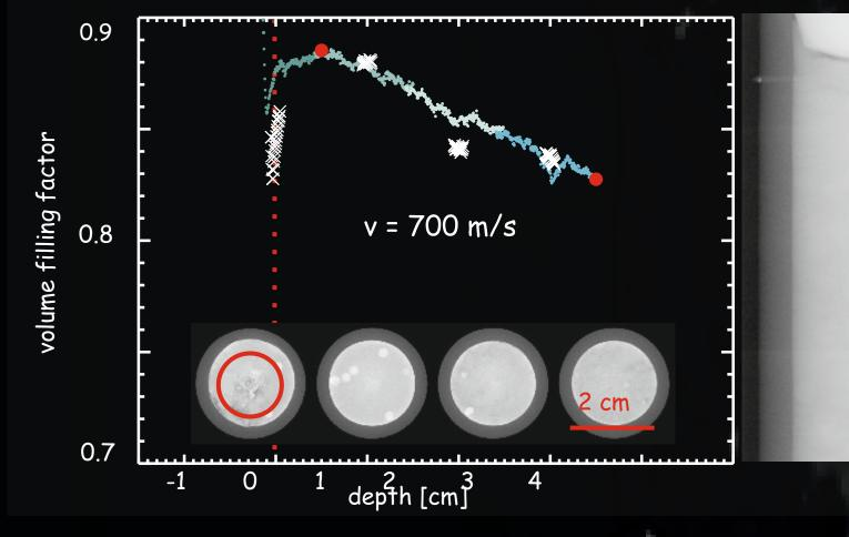
Chondrules start to fragment when the pressure exceeds their respective tensile strength. When the chondrules are in contact to each other, their fragmentation starts at lower pressure, an effect caused by the formation of force chains.
