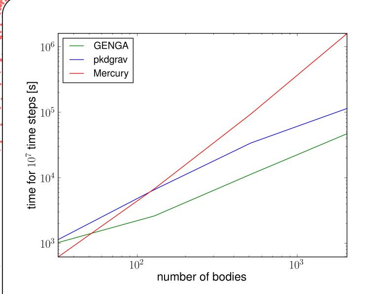
The execution time of GENGA and Mercury scale both with N², but GENGA is up to 30 times faster. Compared to the tree code pkdgrav which scales with Nlog(N), GENGA is up to 4 times faster, but reaches much higher precision in the force computation and energy conservation.
