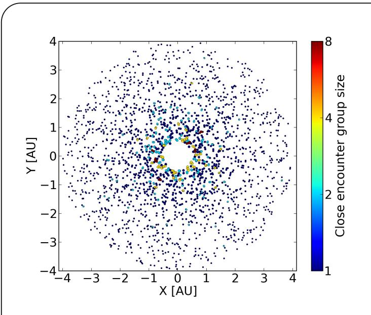
Independent close encounter groups are integrated in parallel with the Bulirsch-Stoer integrator. The close encounter radius depends on the Hill radius and the velocity of the body. Having close encounter groups with too many bodies slows the code down significantly.
