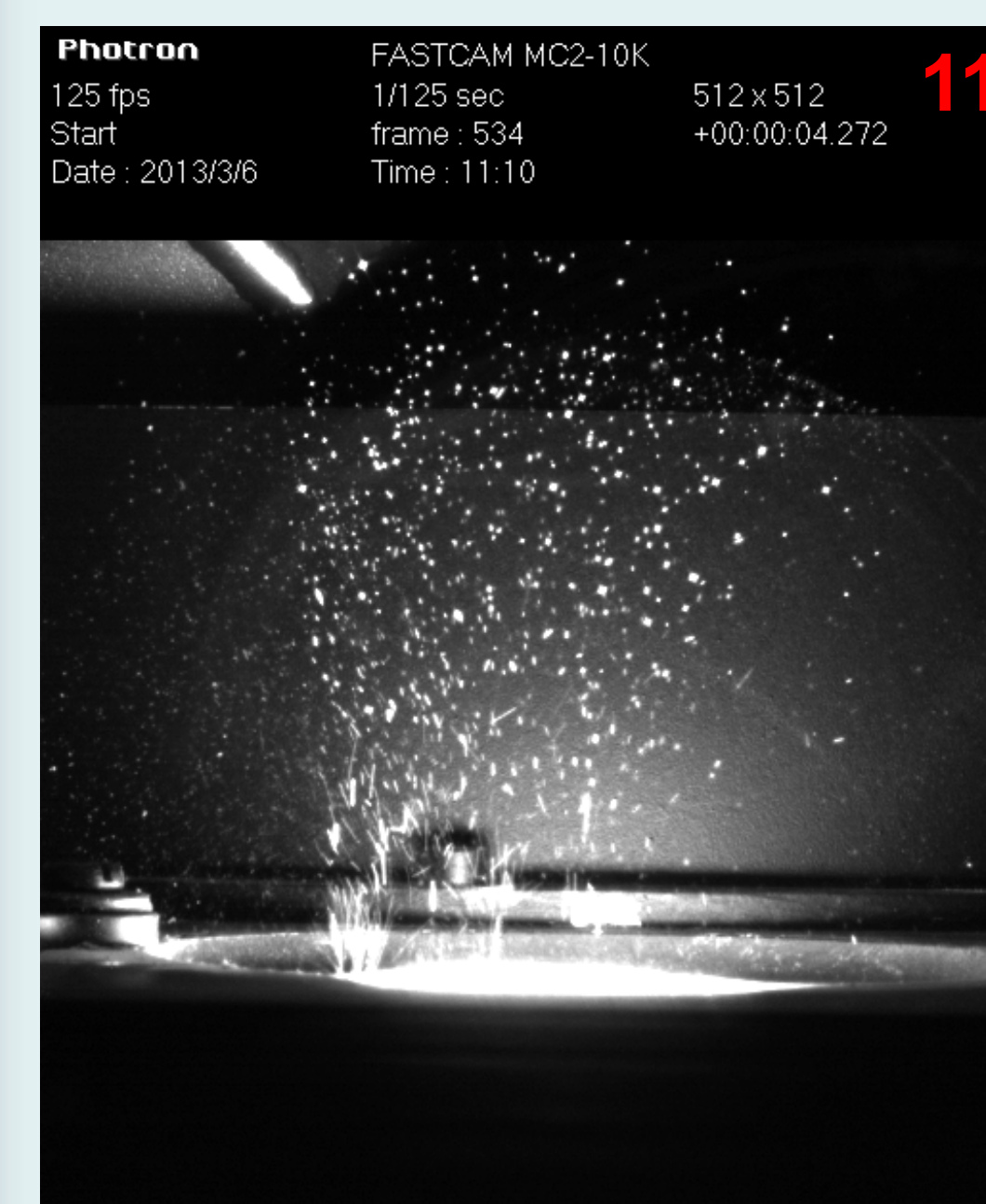
Fig. 11: Snap shot of the eroded particles during microgravity. This frame shows the dust bed of 7 cm diameter from the front (Fig. 10). The lightened part indicates the spot of the IR laser (34 mm spot diameter) upon the dust bed. The light flux is 27 \text{kW}/\text{m}^2 and the ambient pressure is 4 mbar.
