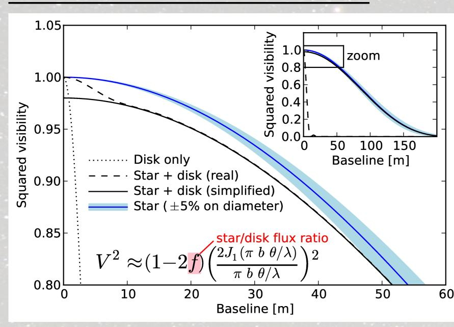
The thermal emission from hot exozodiacal dust (typically several hundred Kelvin up to the sublimation temperature) result in a nearinfrared excess above the stellar flux (typically 1% for known systems). This accuracy is not reachable by simple photometry. It is necessary to spatially disentangle the dust and stellar emission. As the emission
